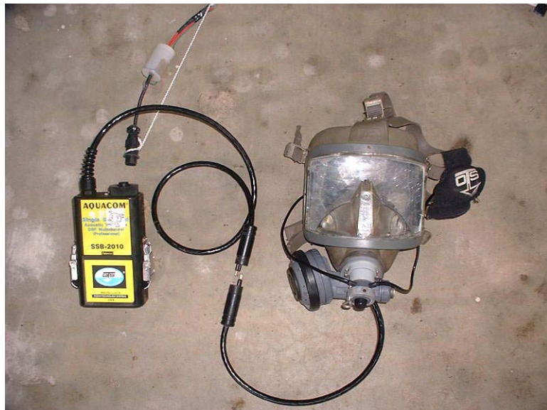
Left: The Underwater Unit, an SSB-2010 with microphone, 2 earphones, and PTT Switch. The inboard end of the antenna with its matching network is visible.
