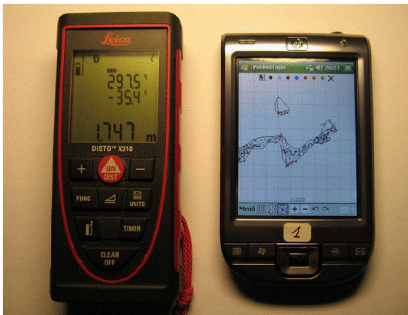
Fig. 2. Leica DistoX2 and PDA with PocketTopo software.
