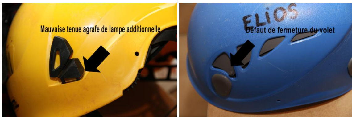
ALVEO and ELIOS, accessories damaged or insecure: frontal fixings, ventilation flaps.
