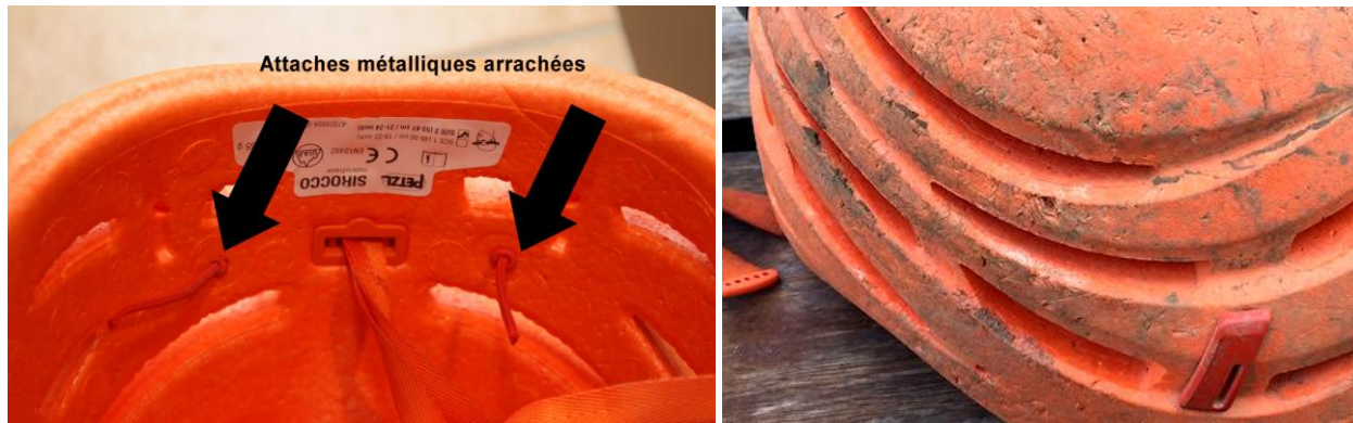
Sirocco : the two tabs of the elastic gave way. Traces of heavy use (only on surface).
